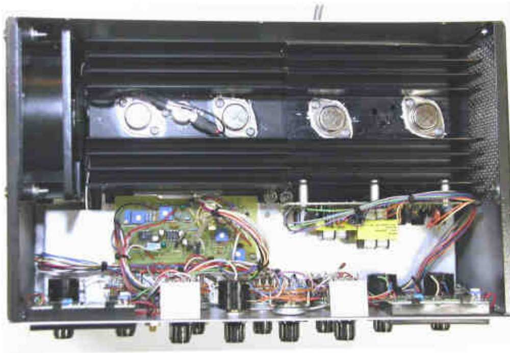
Fig. 12. Top chassis view. Heat sink mounted transistors are at top along with thermal switch. Power supply is vertically mounted to heat sink and Control Board is chassis mounted. Note extensive components and wiring associated with the front panel controls.
