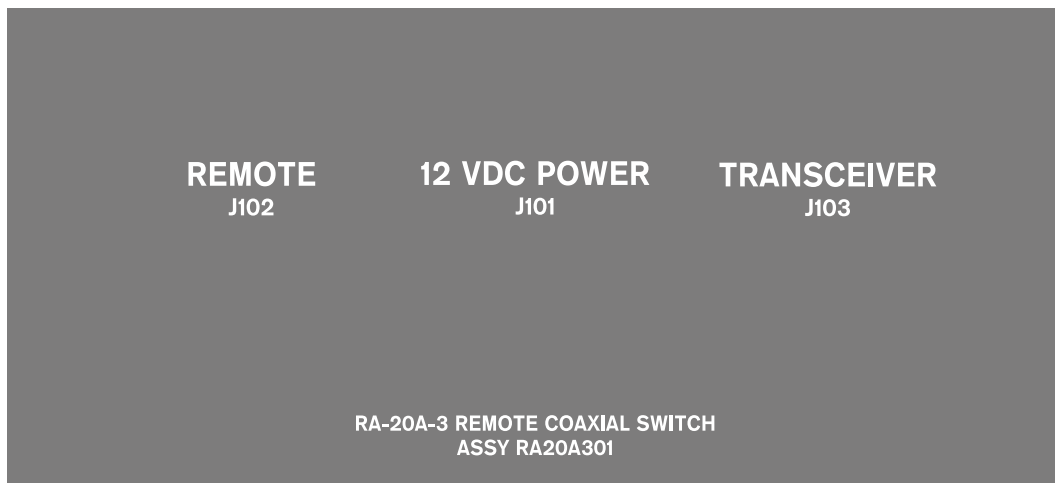
Figure 9. RA20A301 front and rear panel overlays. The rear panel overlay is the same size as the panel, whereas the front panel has additional material to wrap around all edges of the front panel.
