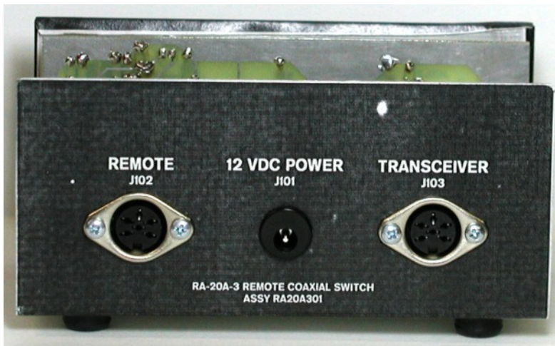
Figure 15 RA20A301 Rear panel showing the connectors.
