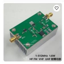
1- 512MHz RF wideband FM power Amplifier 1.6W HF FM VHF UHF RF Amplifier
